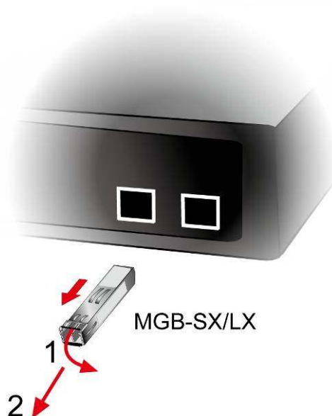
Figure 2-1-2f How to Pull Out the SFP Transceiver
