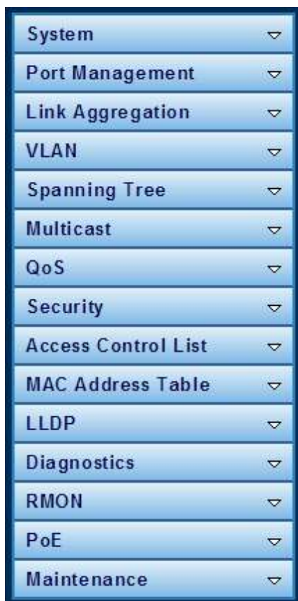
Figure 4-1-5 Managed Switch Main Functions Menu
